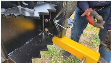
Insert the round tube of the receiver hitch into the square opening underneath the hanger.
