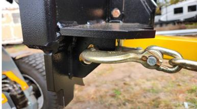
Don't forget to use the chain locks on the grapple hanger to secure your chipper or trailer!
