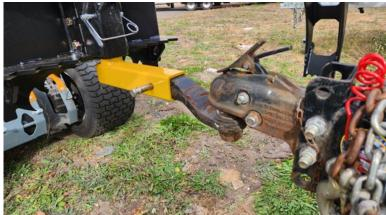
Insert your receiver into the receiver tubing and secure it using a pin.
